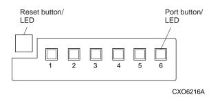
Figure 1–7. HSZ80 Controller Operator Control Panel (OCP)
